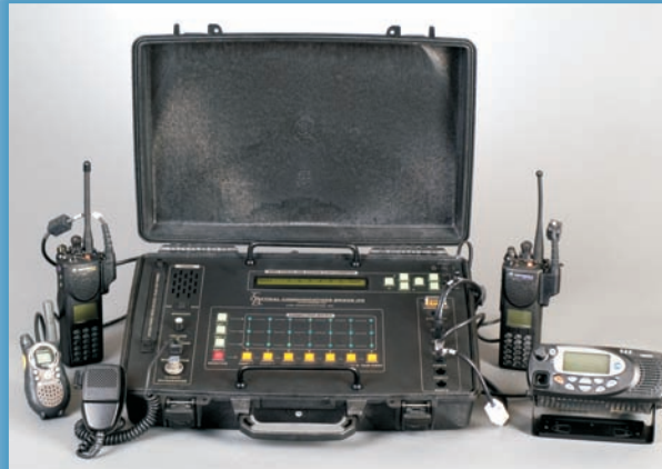
Small Size: Housed in a rugged briefcase enclosure (18" x 12" 4")
