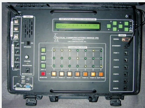
Easy to Use: Front panel operation matrix with simple pushbutton control of 3 Nets plus a User Operator Position
